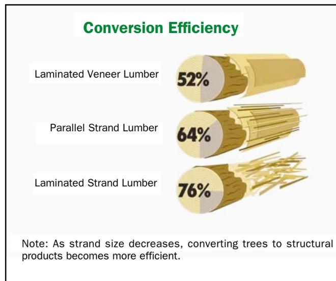
Figure 2 above shows the conversion efficiency of laminated veneer lumber (LVL), parallel strand lumber (PSL), and laminated strand lumber (LSL). These are examples of structural composite lumber (SCL).
